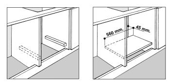
When installing on a built-in oven without forced ventilation, ensure that there are air inlets and outlets for ventilating the interior of the cabinet adequately.
